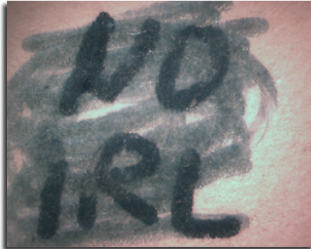
IR Absorption/Reflection reveals obliteration
